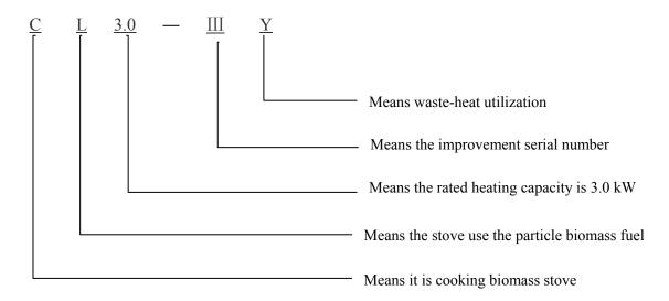
The model above means this kind biomass stove is a cooking stove, the cooking power is 3.0 kW, and can utilize surplus heat.
