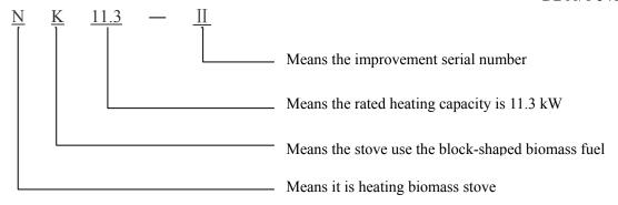
The model above means this kind biomass stove is a heating stove, the rated heating capacity is 11.3.
