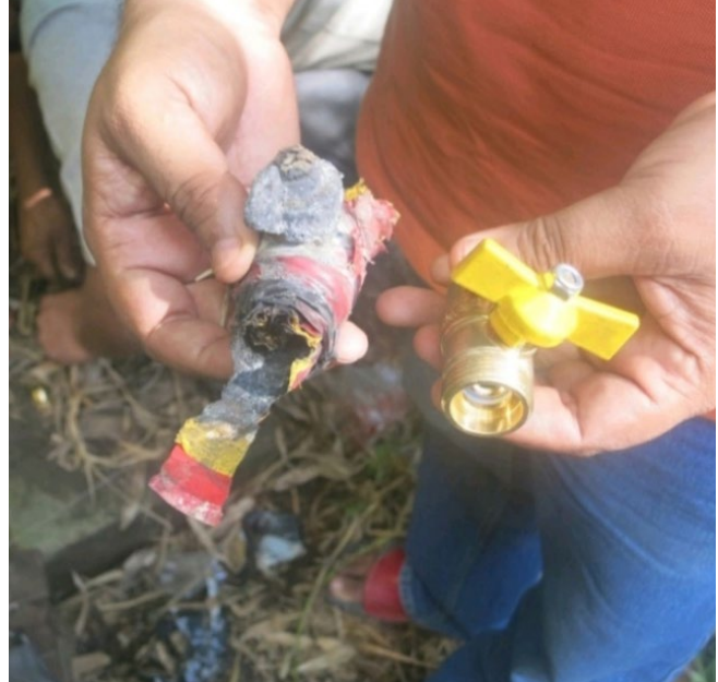
A broken gas valve pictured next to a new valve for comparison.
